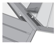
If the roof has a valley, overlap the Kerabit 7 membranes with the valley membrane by 200mm. Cut the ends of the membrane sheets to the line of the valley with the help of a measuring board, and attach them carefully using sealing adhesive along the entire overlapping section. Do not use nails!
