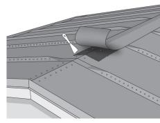
Slice the Kerabit 7 membrane so that you obtain two 350mm wide strips. Attach the strip to the ridge along its entire length using sealing adhesive. The strip laid across the ridge must not be attached with nails. Overlap the extensions by 150mm, attach the end of the lower strip to the substrate using nails with 100mm spacing, and attach the topmost strip to the lower one across the entire overlapping section using adhesive.
