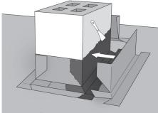
Before installing the roofing, attach a triangle batten at the base of the chimney or other major penetration in order to make the angle less steep. Below and on the sides of the penetration, install Kerabit 7 on the top edge of the triangle batten. Install the membrane above the penetration only after you have completed the upturns of the chimney.
