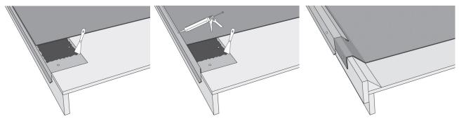
For **verges**, three alternatives exist: Kerabit Eave Flashing, Verge Flashing with ridge, and Verge Flashing. The first two must be installed before the roofing is laid, similarly to the installation of the lower eave flashing. The installation of verge flashing is started from the lower eave towards the ridge.
