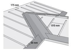
Triangle battens must be approximately 50 x 50mm in size.
