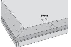
**On the eaves**, Kerabit Eave Flashing is installed. The flashing joints must overlap at least 50mm and be secured with clout nails or sheet metal screws with a KFR head in a zigzag pattern with 100mm spacing. In joints, the drip edge of the uppermost flashing is opened up in order to house the drip edge of the lower flashing.
