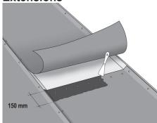
Overlap the membranes by 150mm. Attach the end of the lower membrane sheet to the substrate using nails with 100mm spacing. Attach the top membrane to the lower one across the entire overlapping section using adhesive. In order to obtain a finished seam, use masking tape.
