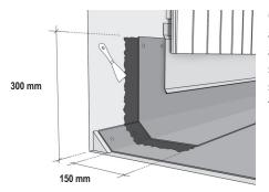
Cut the membrane strips required for the upturn so that they extend at least 30mm up the vertical surface and 150mm over the roofing at minimum. Glue the pieces throughout in place and mechanically secure the fastening of the upturn by nailing. Protect the upturn with sheet metal cladding in order to prevent water from entering between the membrane and the vertical surface.
