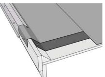
**For verges**, there are three options: Kerabit Eaves flashing, Verge flashing with ridge, and Verge flashing. The first two referred to must be installed as the lower eaves flashings but on verges only in connection with installing the roofing, because the collar of the flashing needs to be installed between the membranes.
