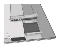
Align the next membrane strip on top of the adhesive surface of the previous strip so that the granulated surfaces meet. The membrane is rolled, nailed, and installed as in the above.
