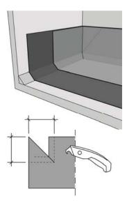
Cut off a triangular piece from the corner of the surface strip, as in the image. The width of the back of the triangle batten strip affects the dimension of the piece to be cut off. Fold the upturn pieces in place, remove the protective plastic cover and, press tightly in place.
