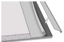
Turn the plastic film covering of the starting strip back and set the eaves flashing of the verge on top of the adhesive surface of the starting strip. Nail the flashing to the underlay in a zigzag pattern at 100 mm intervals. Turn the protective plastic cover back.
