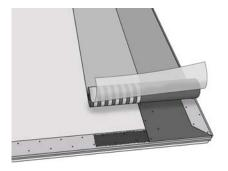
Cut the protective plastic cover on the bottom side of the membrane. Roll out the membrane while simultaneously removing the film and press the membrane to attach it evenly to the starting strip and eaves flashing. Install the other end of the membrane in the same way.
