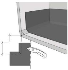
Align the starting strip with the balcony edge so that there is a 300 mm upturned section on the walls. Cut off a piece from the corner of the starting strip, as in the image. The width of the back of the triangle batten strip affects the dimension of the piece to be cut off. Fold the upturn pieces so that they settle to a butt seam at the corner.
