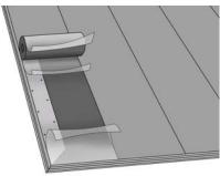
The last strip to be installed is always the end strip with the granulated surface. Do not nail the last strip!
