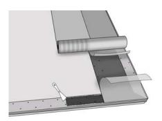
Align the subsequent membrane with the lower and side edges on top of the starting strip. Roll up the aligned membrane halfway back from the lower eaves. Cut the protective plastic cover on the top side of the starting strip, and then remove it for the visible part. Nail the starting strip to the underlay at the edge at 150 mm intervals in a zigzag pattern. Spread an approx. 1 mm layer of sealing adhesive on the flashing of the lower eaves over a width of 500 mm.
