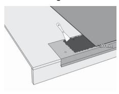
**On lower eaves**, Kerabit Eaves Flashings are installed. The extension points of the flashings are overlapped by at least 50 mm and fixed by felt nails or KFR-headed thin sheet screws at intervals of 100 mm in a zigzag pattern. At extensions, the drip of the topmost flashing is opened and the drip of the lower flashing is installed within the opened one.
