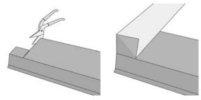
Cut the eaves flashing as shown in the image, put it in place and fold the corner of the metal sheet against the side of the triangle batten strip. Nail the flashing to the underlay in a zigzag pattern at 100 mm intervals. Overlap the extension points of the flashing by 50 mm.
