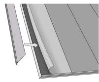
Turn the protective plastic cover of the adhesive surface back, set the eaves flashing of the verge on top of the adhesive surface and nail to the underlay at 100 mm intervals in a zigzag pattern. Turn the protective plastic cover back.
