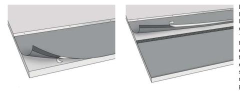
Lay out the membrane in a straight line on the lower eaves and slightly over the edges so that the edges can be folded approximately 15 mm under the lower edges of the boarding. Pre-nail at the top edge at approximately every 1 m through the protective plastic cover of the adhesive strip on the top side. Lift up the lower edge of the membrane, remove the protective plastic cover of the adhesive strip, and press the membrane tightly
