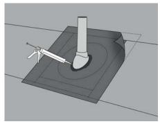
Cut two 1 x 1 m pieces from Kerabit 4000 UT Hitsi. Heat the bottom side of one of the pieces so that the plastic and bitumen mass melt. Press the piece in place over the lead-through opening. Use a knife to cut a hole at the opening. Heat the top surface of the piece at the section that comes under the leadthrough seal, and carefully press the lead-through seal in place. Screw/nail the collar edges and nail the edges of the membrane lay membranes from the pane by
