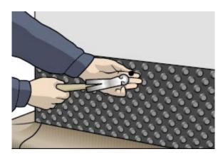
**7.** Fasten the top edge of the foundation panel with plug nails or fasteners at 25 cm intervals. The plate is finally set against the foundation wall by the weight of the soil.
