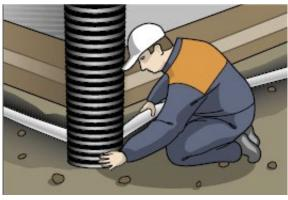
**9.** The functionality of the structure must be ensured using the appropriate filling material, drainage and ground surface gradients away from the building.
