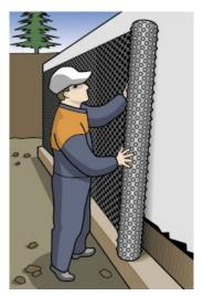
**6.** Cut the foundation panel to the correct height. You can cut the roll with a hand saw to make it narrower. Individual cuts are made using scissors or a carpet knife. When installing the panel, ensure that it is the right way round, with the studs against the foundation wall. This way, an air gap is left between the panel and the foundation.
