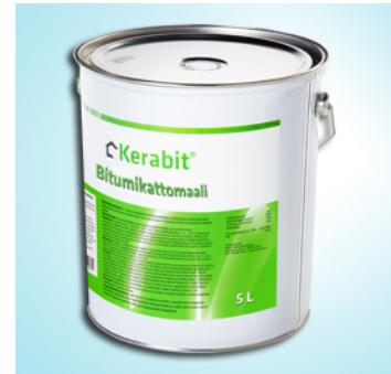
Drying time 3 – 4 hours at +20 °C. Working temperature +5...+25 °C. Bitumen paint is not thinned. Carefully mix the paint before use and during use. If you need more than one container to paint a continuous roof surface, mix all the paint you will need in one container before you start painting so as to avoid colour variation. Clean the surface to be treated from dust, dirt and loose surface particles. Spread the paint with a paintbrush or a broom. Clean the tools with white spirit.
