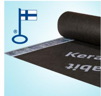
The carrier consists of strong polyester. The top surface of the product is coated with a polypropylene fibre cloth and sand granules at the bottom surface. The 100 mm wide adhesive sections are located on the top and bottom surfaces, on opposing sides.
